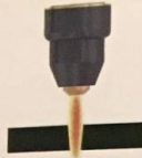
Torch height too high excessive bevel, plasma Stream may not cut all the way through the material
